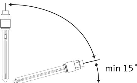
**Figure 3:** Never mount a pH sensor horizontally.
