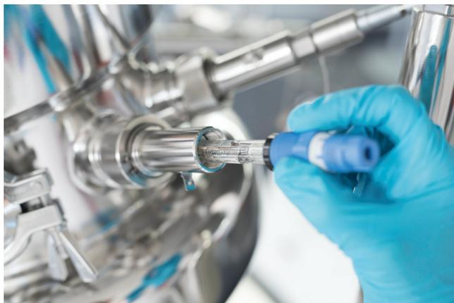
**Figure 2:** Glass pH sensors are fragile. Handle carefully.
