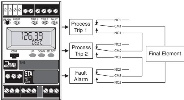
**High Integrity Architecture**—This configuration offers the highest trip integrity in a non-redundant application (Figure 4). Since all three relays are wired in series, any trip alarm or fault alarm will trip the final element or logic solver.
